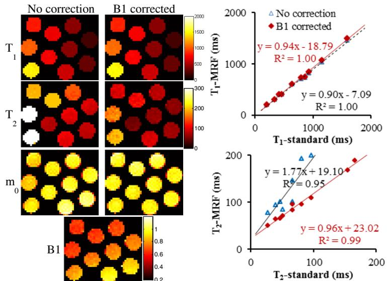
**Fig. 1.**  $T_1$ ,  $T_2$ , and proton density ( $m_0$ ) maps of a water phantom before and after B1 correction. Significant changes in  $T_2$  values were observed after the B1 correction, which is in good agreement with standard values.
