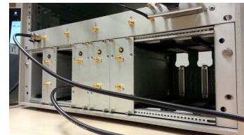
Fig.3: RF feed network components integrated into a 19" rack.
