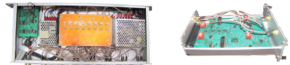
Fig. 2: Final design of the Power divider (left) and one of the modulator cassettes (right).
