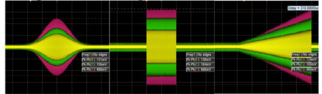
**Figure 2:** Shaped RF pulses with various amplitude and phases at the output of Module 1 (green and yellow) compared to RF input signal (in magenta).
