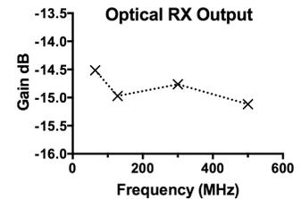
**Figure 4:** Gain of the carrier signal at the optical RX side referred to the amplitude of the input carrier signal.
