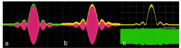
**Figure 3:** Envelope detection before and after modulation optical transmission and demodulation & carrier recovery.
