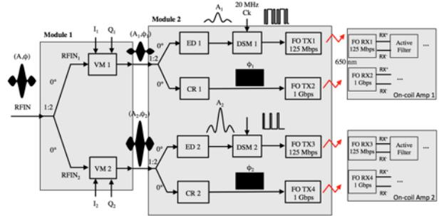
**Figure 1:** Schematic diagram of the modular interface
