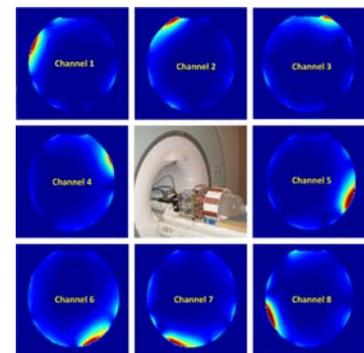
Figure 3. MR experimental setup (center) with a phantom and GRE images of each channel.
