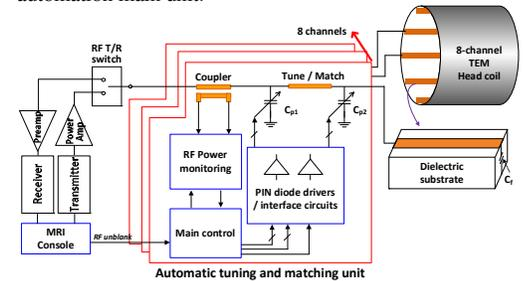
Figure 2. The block diagram of automatically tuned and matched 8-channel RF transceiver coil for 7T.
