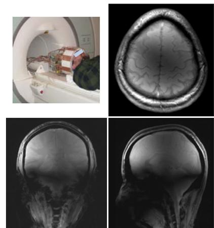
Figure 4. Human head images obtained with the automatic tuned and matched RF coil at 7T.
