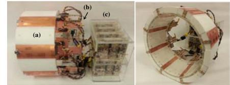
Figure 1. Automatically tuned and matched RF transceiver head coil. (a) TEM coil elements, (b) electrically controlled capacitor arrays and couplers, and (c) an automation main unit.
