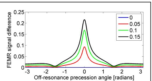
**Fig. 2:** Results of a Bloch-equation simulation, showing the magnitude of the coherent FEMR signal difference as a function of off-resonance precession angle, for several ARFI-induced phase angles (given in radians).  $T_1 = 900$  ms,  $T_2 = 90$  ms,  $TR = 10$  ms, and flip angle =  $20^\circ$  were assumed.
