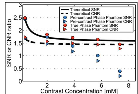
**Figure 1:** SNR and CNR ratios of Dixon vs. Subtraction CE-MRA within the phantom. Results are shown using pre-contrast phase and true phase in the Dixon reconstruction.
