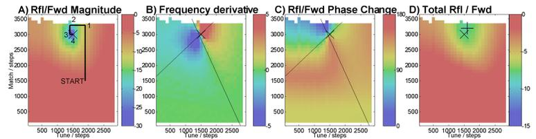
**Fig. 1:** Evaluating 4 possible optimisation metrics on a volunteer at isocentre for a single element of the array coil. Similar features were observed on all other channels and with a phantom at isocentre and outside the magnet. The path taken by the auto-tune algorithm is marked in (A). The lines of maximum gradient in (B) and (C) are marked on both plots. The  $S_{nn}$  minimum is denoted 'x' and in (D) the  $\sum_m S_{nm}$  minimum is denoted '+'.
