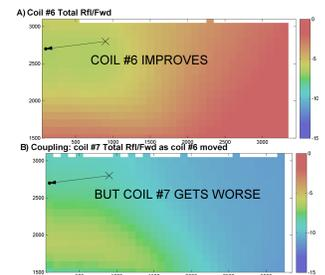
**Fig. 2:** Effect of adjusting coil #6 on total reflected power (ie. coupling).
