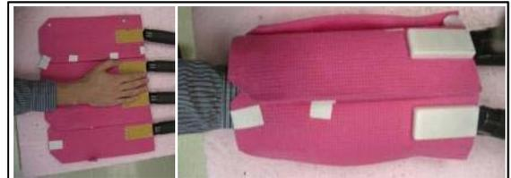
**Figure 1: Unilateral 8ch receiver coil array. 8 linear elements arranged circumferentially around the hand/wrist**
