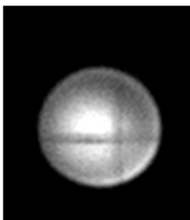
figure 4. One slice from three orthogonally acquired slices of a phantom. Note the saturated cross originating from the other slices, demonstrating accurate slice selection.
