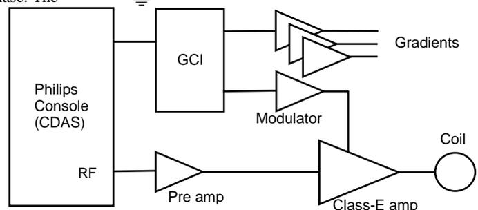
figure 2. Block schematic
