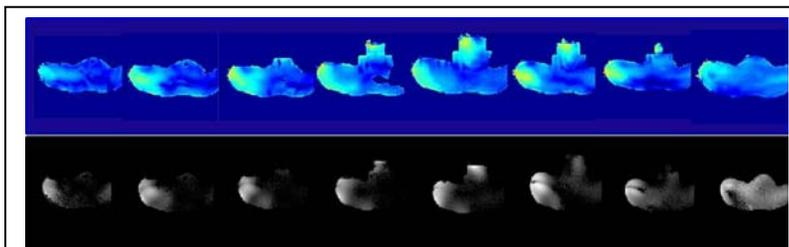
**Figure 2.** (Top) Optimized B1+ maps throughout homogeneous human body phantom and (bottom) corresponding experimental data obtained at 7 Tesla
