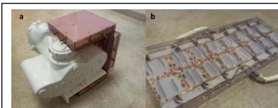
**Figure 1.** Assembled a) 12-Ch Transmit Body array and b) 16-channel Receive insert.
