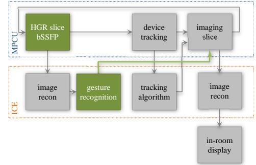
**Fig. 1:** Flow diagram of an interventional pulse sequence (gray) extended by a hand gesture recognition (HGR) slice acquisition on the scanner (MPCU) and the HGR algorithm (green) on the image reconstruction system (ICE).
