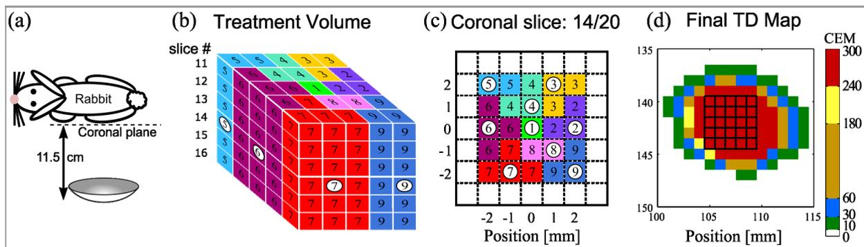
**Figure 1:** [a] Experimental setup, [b] controller configuration: 3D treatment volume (circled #'s indicate focal zone center and order), [c] controller configuration: central 2D slice through 3D volume, [d] final thermal dose map through central treatment slice.
