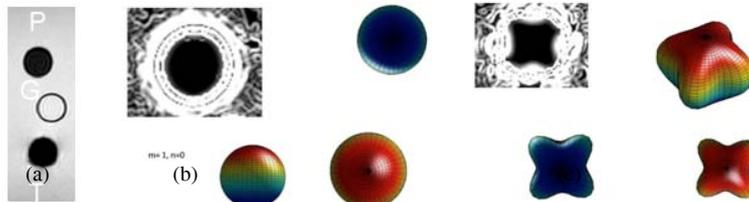
Figure 1. (a) mFFE image of the three phantoms. (b)Magnetic field simulated projection with vibration mode with m=1 and n=0. (c)Projection of the magnetic field and vibration mode of the electrical field inside the sphere.
