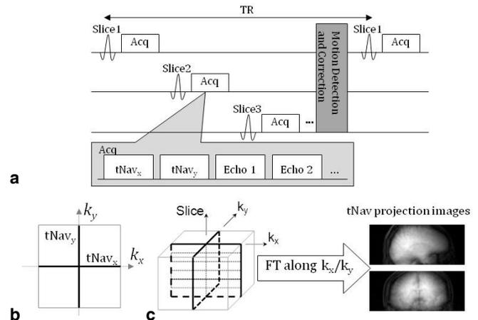
**Figure 1** The scheme of tNav. (a) Two tNav echoes are inserted into the acquisition window of each slice. Real-time motion detection and correction is carried out at the end of each TR. (b) Two tNav echoes sample the  $k$ -space of each slice along the  $k_x = 0$  and the  $k_y = 0$  lines. (c) After an inverse FT is taken along  $k_x/k_y$  direction, two orthogonal tNav projection images are reconstructed for through-plane motion detection.
