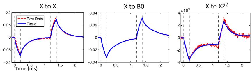
Fig. 2. Top three EC components from analysis of a HOEC dataset acquired on a GE 3T scanner with a 21-cm spherical phantom. Vertical axis represents the coefficients after the polynomial fitting.
