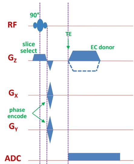
Fig. 1. Pulse diagram of the short term HOEC measurement sequence.
