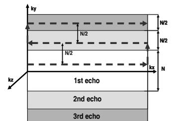
Fig. 1 Example of a turbo=3 acquisition scheme. The dashed line illustrates a k-space trajectory traversed after a single excitation.
