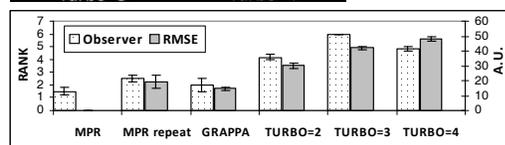
Fig. 3 Observer ranking and RMSE (with respect to the MPR) of the different scans averaged across subjects. Error bars show standard deviation as error estimation.
