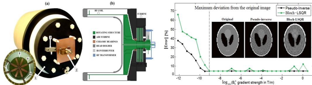
**Fig.1** – (a) Photograph and (b) side view of the rotating RF coil (RRFC) system consisting of (1) air turbine, (2) the inductively coupled RF link, (3) infrared photo-interrupter, (4) RF coil, (5) PCB and (6) tuning capacitor.
