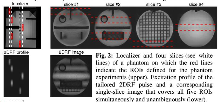
**Fig. 2:** Localizer and four slices (see white lines) of a phantom on which the red lines indicate the ROIs defined for the phantom experiments (upper). Excitation profile of the tailored 2DRF pulse and a corresponding single-slice image that covers all five ROIs simultaneously and unambiguously (lower).
