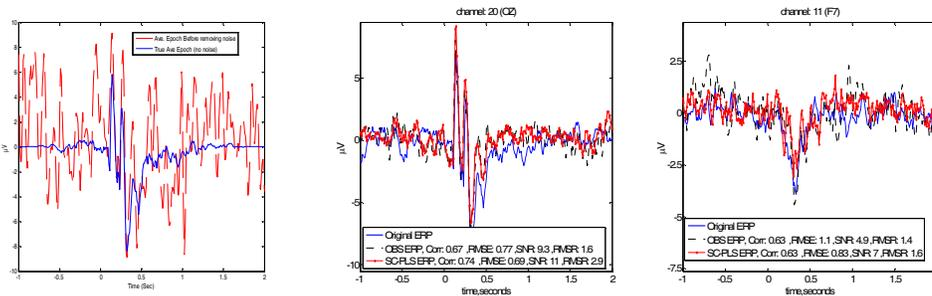
**Figure 1:** Left: ERP from EEG collected outside (blue) and inside MRI (red). Middle and right: ERP signal obtained after cleaning the noisy EEG using OBS method (dashed) and SC-PLS (red) compared to the reference ERP (Black) for channels OZ and F7.
