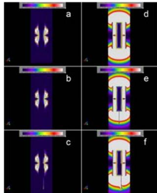
**Figure 3**  $\vec{E}$  field magnitude in the coronal slice through the conductive wire. (a) LTx no wire (b) LTx wire centered (c) LTx wire off-center (d) WBC no wire (e) WBC wire centered (f) WBC wire off-center. Scale: 15 V/m - 75 V/m
