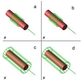
**Figure 1** Configurations of the simulations described. (a,b) LTx coil 40cm diameter, 50cm length; (c,d) WBC 60cm diameter, 130cm length. (a,c) wire centered; (b,d) wire off-center.
