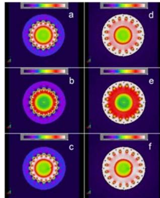
**Figure 4** Rotating  $\vec{B}_1^+$  field in the axial slice through isocenter. (a) LTx no wire (b) LTx wire centered (c) LTx wire off-center (d) WBC no wire (e) WBC wire centered (f) WBC wire off-center. Scale: 0 $\mu$ T - 2 $\mu$ T
