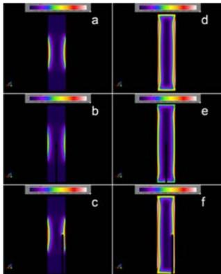
**Figure 2** Graphical display of SAR (raw) in the coronal slice through the conductive wire. (a) LTx no wire (b) LTx wire centered (c) LTx wire off-center (d) WBC no wire (e) WBC wire centered (f) WBC wire off-center. Scale: 0 W/kg - 2 W/kg
