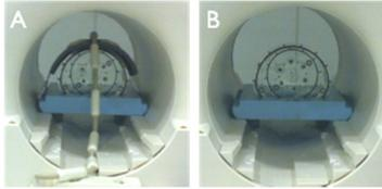
Fig. 1: Phantom setup: NEMA phantom was placed in the PET FOV without the patient table and was scanned with (A) and without (B) the local RF coil.
