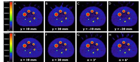
Fig. 5: PET FBP images for different shifts and rotations between  $\mu$ -map and real position of the RF coil showing the artifacts in the region of the RF coil.
