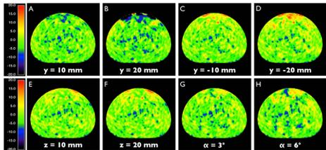
Fig. 4: Difference images of the PET OSEM images for different shifts and rotations between  $\mu$ -map and real position of the RF coil (range -20% to 20%).
