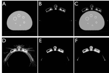
Fig. 2: Transaxial slice of following CT-based  $\mu$ -maps: (A) phantom (human  $\mu$ -map), (B) RF coil (hardware  $\mu$ -map), and (C) overall  $\mu$ -map. CT-based  $\mu$ -map without (D) and with post-processing (E) and with Gaussian filter and threshold (F). (Note: window width is changed to display the noise)
