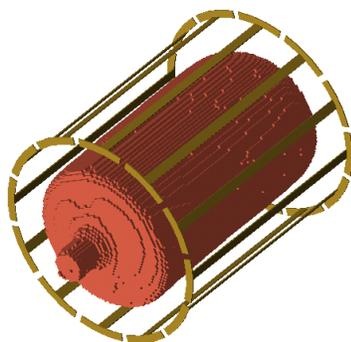
FIG.1. Simulation and experimental setup of a cylindrical phantom inside an extremity birdcage coil.
