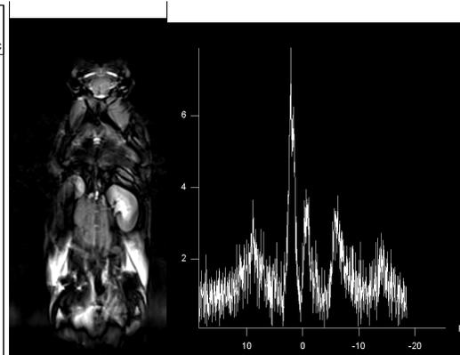
Fig.3: T2- weighted TSE image of a living mouse and 31P-spectrum measured with PIN-Diode -BC
