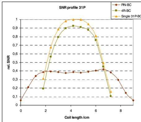
Fig.2: 31P- SNR profile of the selected coils along the coil axis.
