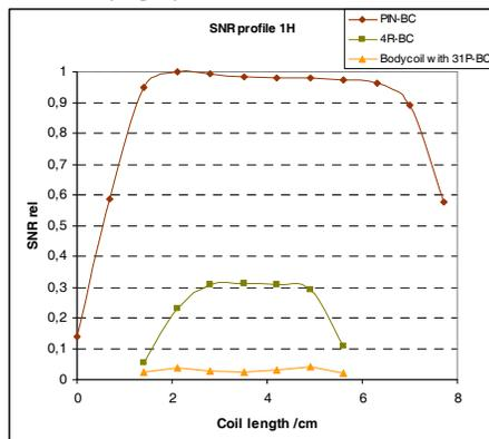
Fig.1: 1H- SNR profile of the selected coils along the coil axis.
