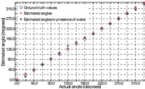
Fig. 5: Rotor angle estimation in the absence and presence of water.
