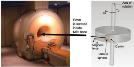
Fig. 1: MR-powered actuator concept.
