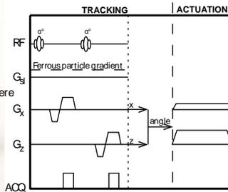
Fig. 4: Pulse sequence for tracking and optimal gradient generation.
