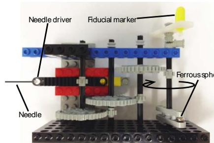
Fig. 2: The MRI-powered actuator on a needle driving robot.
