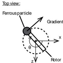
Fig. 3: Orthogonal gradients supply max torque.
