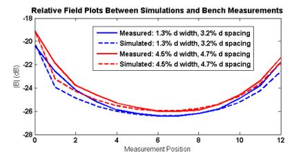
**Figure 3:** Relative field plots comparing modeling results and bench measurements for  $|B|$  across the plane of the unloaded coil plane. The measured and simulated data for each test case largely agrees throughout the coil's excitation region.
