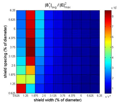
**Figure 2:** Color-weighted plot illustrating the ratio of  $|B_1^+|/|E|^2$ . Note the second column shows a parameter region with more desirable improved field effects.
