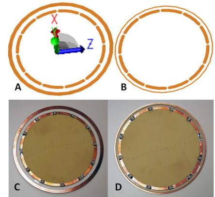
**Figure 1:** Two software renderings and constructed coils with co-planar shields. **A:** 7mm width shield spaced 8mm from the coil conductor (representing 4.5% coil diameter width and 4.7% diameter spacing). **B:** 2mm width shield spaced 5mm from the coil (1.3% diameter width and 3.2% spacing). **C-D:** corresponding coils used for bench testing, respectively.
