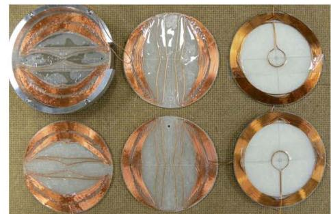
Fig.3 Coil elements for the 40 mm bore probe
