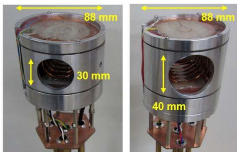
Fig.1 Gradient probes (bore = 30 and 40 mm)
