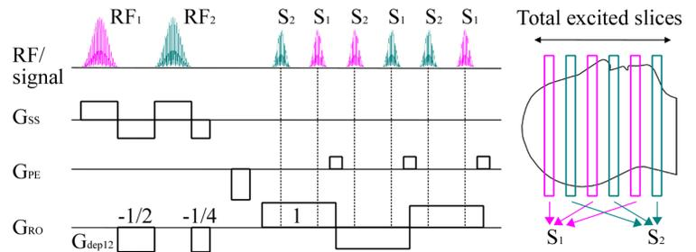
**Figure 1** An M-EPI sequence diagram and its slice-excitation profiles used in this study. The value put on the gradients in the GRO direction represents the relative momentum of the gradients. The RF<sub>1</sub> and RF<sub>2</sub> are generated by applying a sinusoidal modulation to a sinc RF pulse and excite three slices simultaneously marked by S<sub>1</sub> and S<sub>2</sub>, respectively.
