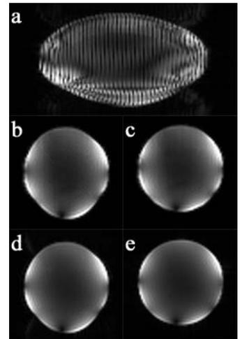
**Figure 2** Oil phantom images at 9.4T (a) an image from 2D FT reconstruction of the M-EPI data, (b) a representative slice from M-EPI reconstruction of the M-EPI data, (c) the distortion-corrected version of (b), (d) a single-shot EPI and (e) a gradient-echo image at the same slice position.
