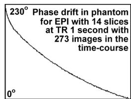
**Fig.1.** B<sub>0</sub> drift of ~22 Hz for EPI of the phantom.
