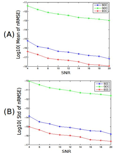
**Figure 3 (in color):** (A) mean and (B) standard deviation of nRMSE of combined images from compressed channels as a function of SNR.
