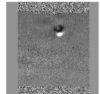
Figure 2.  $\mu$ MRE wave image from a set of 240 acquired from the bottom slice of an agarose gel phantom at 156 x 125  $\mu$ m resolution over a 6.4 x 6.4 cm FOV. Animations show complex wave behavior at the soft gel occlusion.
