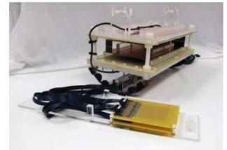
Figure 1. Insertable 64 element planar pair receive array in a “sandwich” configuration shown with non-linear gradient coil and integrated RF volume excitation coil.
