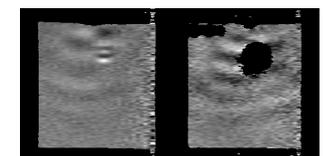
Figure 3. SEA MRE wave images from a set of 240, each echo simultaneously acquiring images at the bottom (left) and top (right) slices of the phantom, with the entire set acquired in 4 minutes. The non-linear gradient was employed for RF phase compensation.
