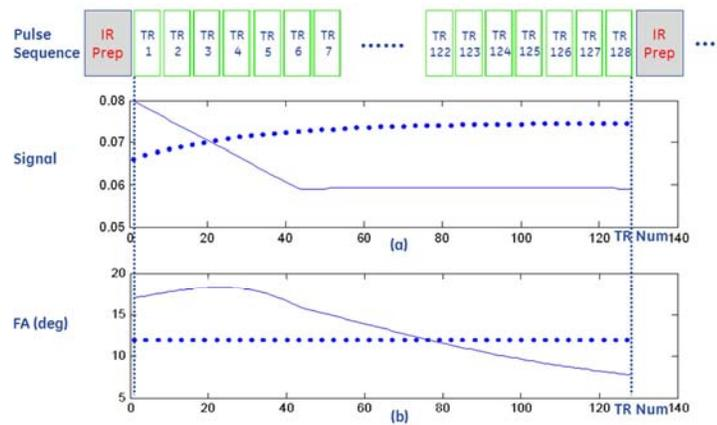
**Figure 2:** In an IR prepared SPGR, a fixed FA scheme (dotted line in b) will lead to an increasing signal in consecutive TRs. The FANS-designed variable FA scheme (solid line in b) leads to a signal modulation that is high at beginning and then drops (solid line in a), which achieves better CNR in practice.
