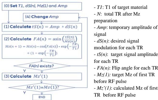
**Figure 1:** Block diagram of the procedure to implement FANS algorithm. By setting different  $Mz(1)$  and  $dS(n)$ , the signal for each TR is changed, which can be used to tune image quality.
