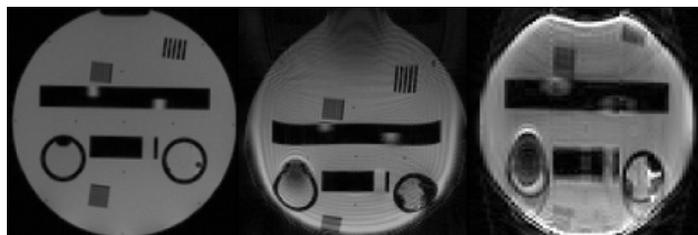
**Fig. 2:** Axial images obtained from a structural water phantom with 3D FLASH (left), 2D EPI (middle) and 3D center-out EPI with cylindrical encoding (right).
