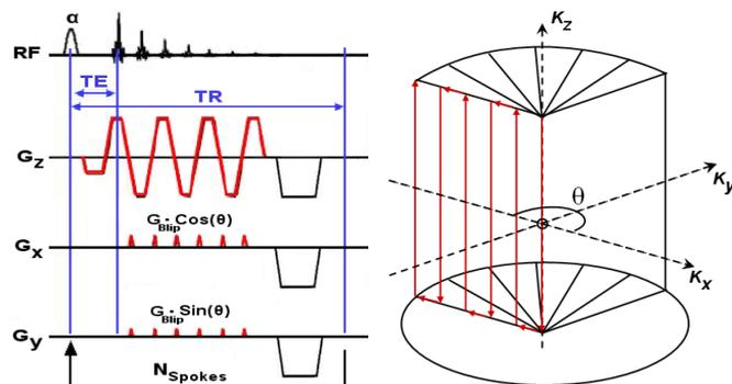
**Fig. 1:** Schematic diagram of 3D center-out EPI with cylindrical encoding (left) and the corresponding  $k$ -space trajectory (right).
