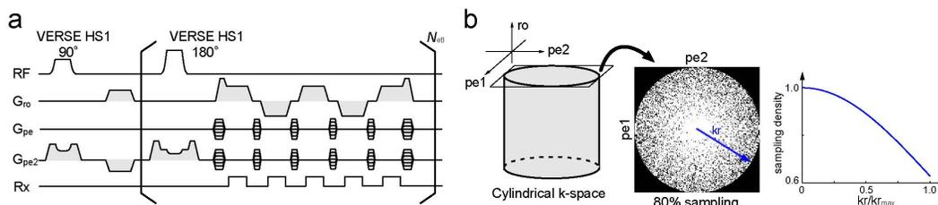
Figure 1. Sequence diagram of the 3D adiabatic FSE sequence (a) and k-space undersampling strategy (b).
