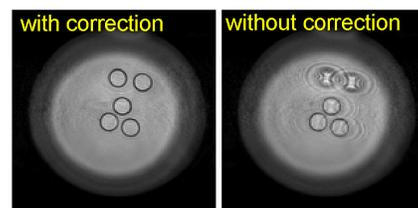
Figure 2. Phantom images reconstructed with (left) and without (right) image space phase correction. ( $T_{E,eff}=25$  ms,  $TR=500$ ms,  $N_{eff}=8$ ,  $tf=5$ , 1min 30sec)
