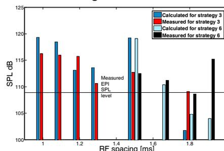
Figure 2. Measured SPL of pCASL labeling module and EPI readout module
