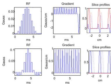
**Fig. 1 – Method A:** Excitation (top) and refocusing (bottom) RF (left), gradient (middle), and resulting slice profiles (right) for the first method. Profile legend: water (full line), fat (dashed line), real (blue) and imaginary (red). Average gradients are 0.23G/cm for excitation and refocusing respectively.
