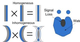
**Fig. 4 – Method B:** Magnetization profile resulting from the second method. By matching the mean slice selection gradient of both RFs, identical slice bending is observed for the excitation and refocusing profiles in the presence of off-resonance.
