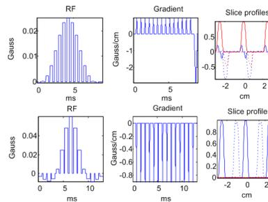
**Fig. 3 – Method B:** Excitation (top) and refocusing (bottom) RF, gradient, and resulting slice profiles for the second method. Profile legend: water (full line), fat (dashed line), real (blue) and imaginary (red). Average gradients are 0.15G/cm for both excitation and refocusing.
