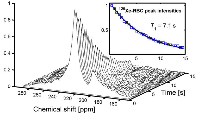
**Figure 1:** Decaying spectra from <sup>129</sup>Xe dissolved in blood acquired with 500 μs hard pulses (TR = 0.5 s) on a 1.5 T scanner. The peaks at ~ 196 and 220 ppm correspond to <sup>129</sup>Xe dissolved within plasma and RBCs, respectively. The inset shows an exponential fit performed on the decreasing <sup>129</sup>Xe-RBC NMR signal to establish a value for <sup>129</sup>Xe-RBC T<sub>1</sub> (fit is for a sample with 0.91 sO<sub>2</sub> and Hct of 57 %).
