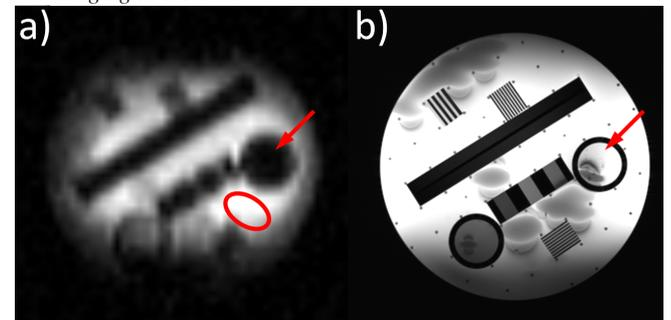
Figure 2: a)  $^{17}\text{O}$  image of the resolution phantom. The red ellipse depicts the ROI for SNR calculation b) Corresponding  $^1\text{H}$  image. The oil-containing vessel (red arrow) is only visible in the  $^1\text{H}$  image as it contains no oxygen.
