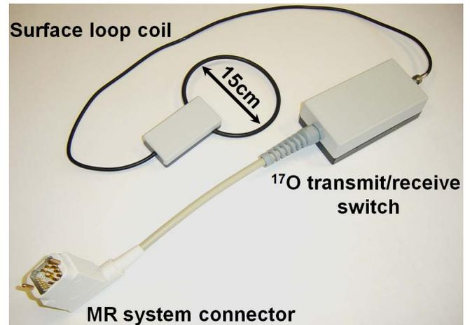
Figure 1: Complete setup of the TxRx switch and surface coil for  $^{17}\text{O}$  imaging at 3 Tesla.
