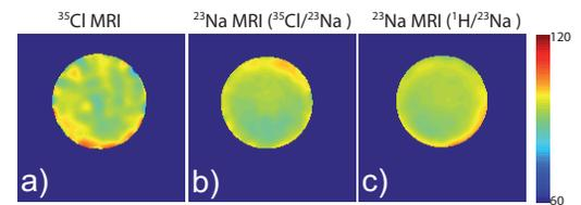
**Fig. 1:** Transversal  $B_1$  maps of the  $^{35}\text{Cl}/^{23}\text{Na}$  coil (version 1) (a, b). a)  $^{35}\text{Cl}$  channel. b)  $^{23}\text{Na}$  channel. c) Transversal  $B_1$  map of the  $^1\text{H}/^{23}\text{Na}$  coil. All setups showed good  $B_1$  homogeneity. Average flipangles in the presented transversal slices: a)  $93^\circ \pm 3^\circ$ ; b)  $93^\circ \pm 3^\circ$ ; b)  $93^\circ \pm 2^\circ$ .
