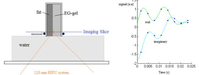
Fig. 2 a) Experimental setup of the HIFU sonication of the fat/EG-gel interface and b) example fits of the real and imaginary signal.
