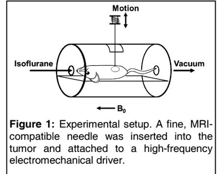
**Figure 1:** Experimental setup. A fine, MRI-compatible needle was inserted into the tumor and attached to a high-frequency electromechanical driver.
