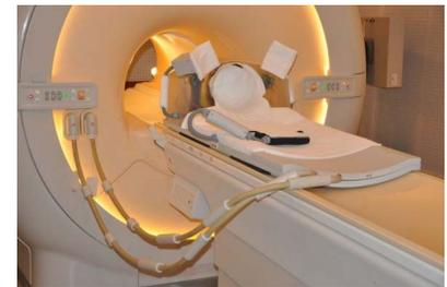
Figure 1: The dedicated 36-channel neurovascular coil.
