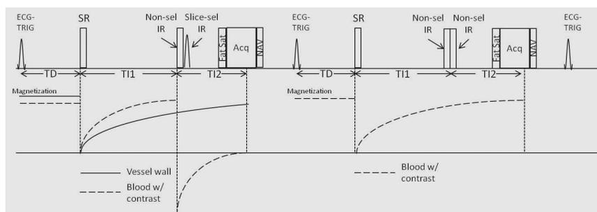
**Fig. 1** Sequence diagram of the ECG-triggered and navigator-gated SR-DIR prepared RF spoiled GRE sequence. Black-blood and bright-blood images data are collected in an interleaved fashion. Blood signal is suppressed by a combination of SR and dual-IR. SR: saturation recovery; IR: inversion recovery.
