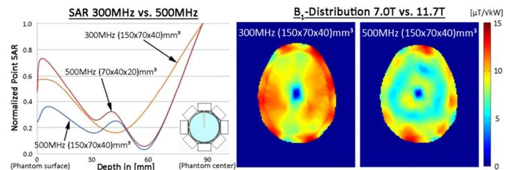
**Figure 3:** Comparison of the target RF-Heating capabilities of three 8ch hardware configurations at 300MHz and 500MHz (left). Comparison of the B<sub>1</sub> distribution at 7.0T and 11.7T with an in-phase phase setting (right).
