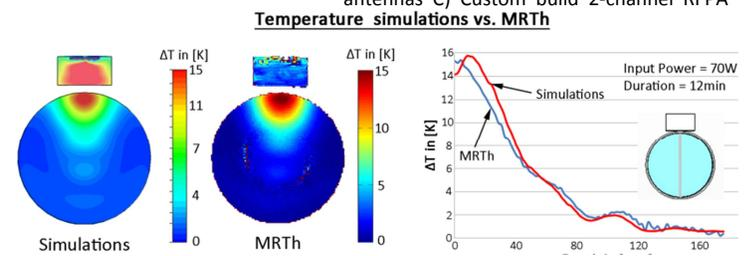
**Figure 2:** Comparison of the results of the simulated temperature distribution of a single antenna at 500MHz in an axial slice of a cylindrical phantom versus MRTh measurements for 70W input power and an RF-Heating duration of 12 minutes.
