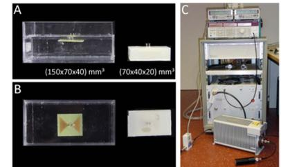
**Figure 1** Hardware for RF-Heating experiments at 500MHz. A-B) Bowtie antennas C) Custom build 2-channel RFPA
