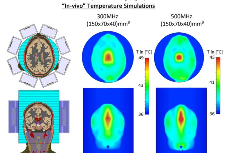
**Figure 4:** Temperature increase induced by a 300MHz and a 500MHz 8 channel bowtie antenna array after 5min of 50W avg power per channel. Temperature change is shown for an axial (top) and coronal (bottom) slice of "Ella". A water bolus was used for cooling purposes and EMF coupling to the brain.
