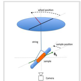
**Figure 1.** The experimental setup, placed in the center of the magnet. The sample in a tube is suspended by a string from a movable wheel. The angle of the wheel and the tube can be observed in real time (and recorded) with the camera placed below the device.
