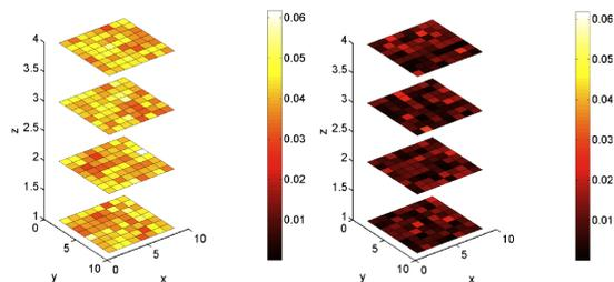
Fig 2: Voxel-wise RMSE between ground-truth and reconstruction obtained for an SNR of 20 by either the SRR by [1] (left) or the proposed SRR (right)
