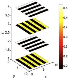
Fig 2: Synthetic phantom: Black voxels mimic grey matter with  $f=0$ . White and yellow voxels mimic white matter with fibre orientations along the x or y axes, respectively
