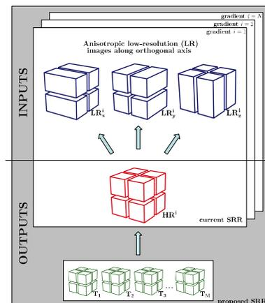
Fig 1: Forward models of the current and the proposed SRR
