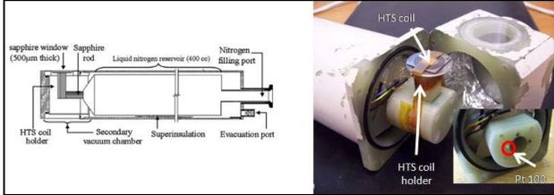
**Fig. 1 :** Dedicated LN<sub>2</sub> cryostat schematic (left), and a detailed view of the HTS coil mounted onto a sapphire cold finger into the secondary vacuum chamber of the cryostat (right). Inner parts of the cryostat body are covered with a superinsulation layer except close to the HTS coil.
