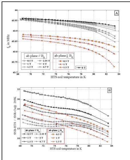
**Fig. 2 :** effects of cooling temperature and field on resonance frequency(A) and on SNR gain for both along and orthogonal orientation with B<sub>0</sub>(B)
