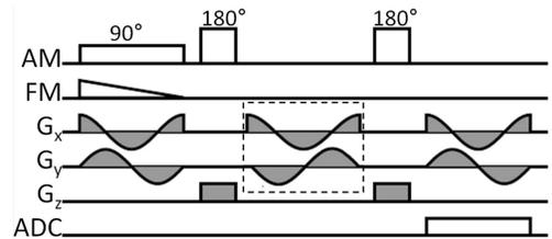
**Figure 1** – STEREO implemented as a double SE. A chirp pulse is used for excitation in the presence of a modulated gradient. Signal is refocused and then acquired. TE is constant across the image. The gradient shapes within the dashed box are optional, but can be used to balance asymmetries in the gradient ramps.
