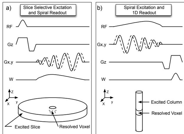
Figure 1: A slice selective spiral pulse sequence (left) can be reversed to form a column selective, 1D resolved pulse sequence.  $W$  is the reconstruction weighting, which becomes the RF pulse when reverse. One resolved voxel is exactly the same with both pulse sequences. Other voxels can be resolved in the readout dimensions.
