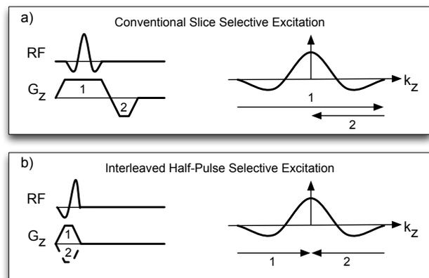
Figure 2: Conventional slice selective excitation (a), and an interleaved half pulse excitation (b).
