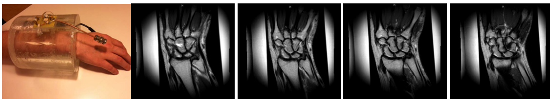
Figure 6. (left) A quadrature HEM_{11} resonator with two inductive coupling loops used for impedance matching. (right) Adjacent slices from the human wrist using the water-based cavity resonator.
