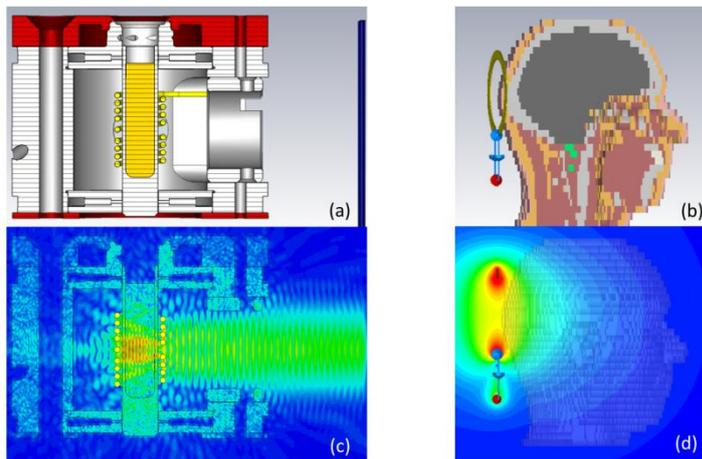
*Figure 1:* Geometrical cross sections through example structures (a) and (b) and numerically computed magnetic field distributions in magnitude representation (c) and (d) at frequencies of interest (263 GHz and 114 MHz, respectively).
